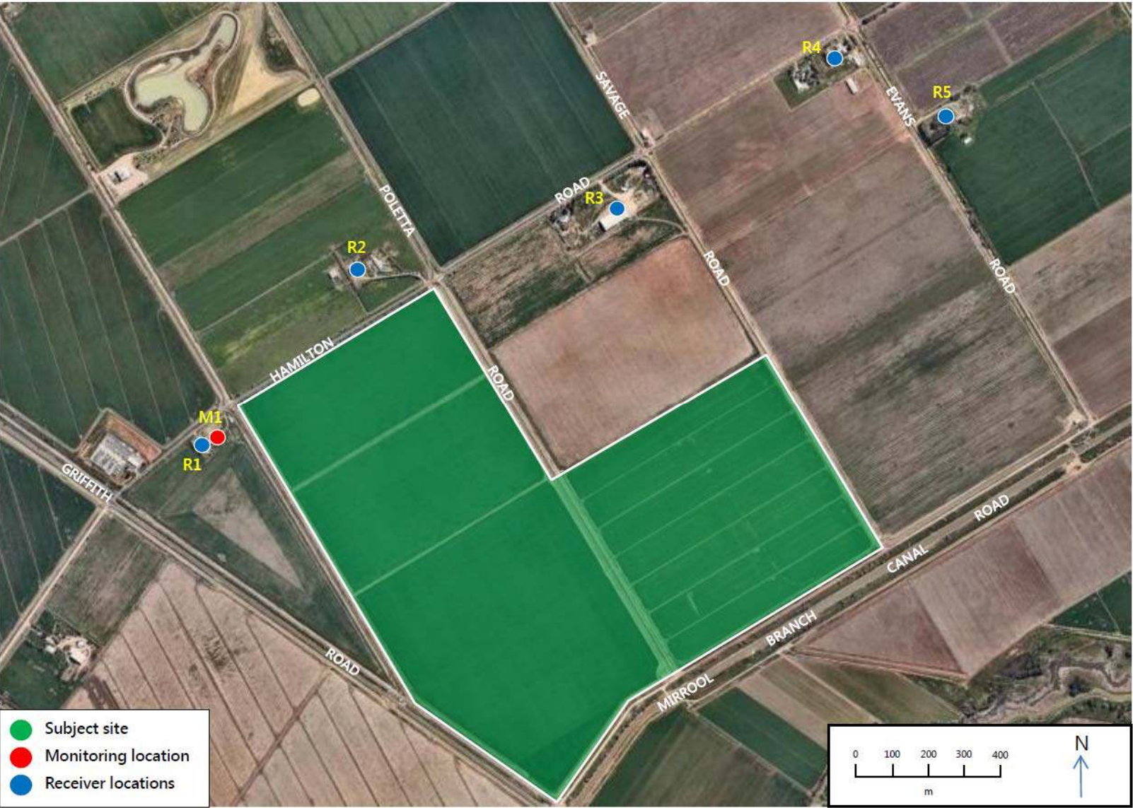
Figure 6-9 Residential receivers and noise monitoring locations adjacent to the proposal site
